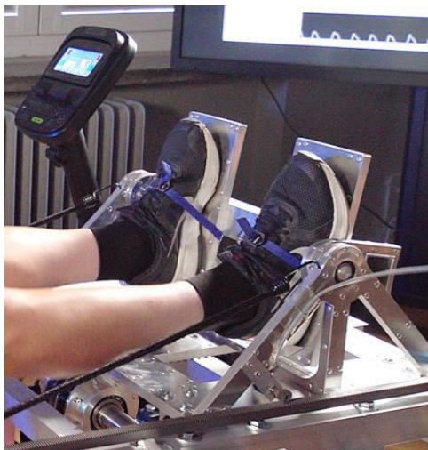
Dynamic tests of the gantry drive in comparison with the crankset were carried out on custom-built test stands.
