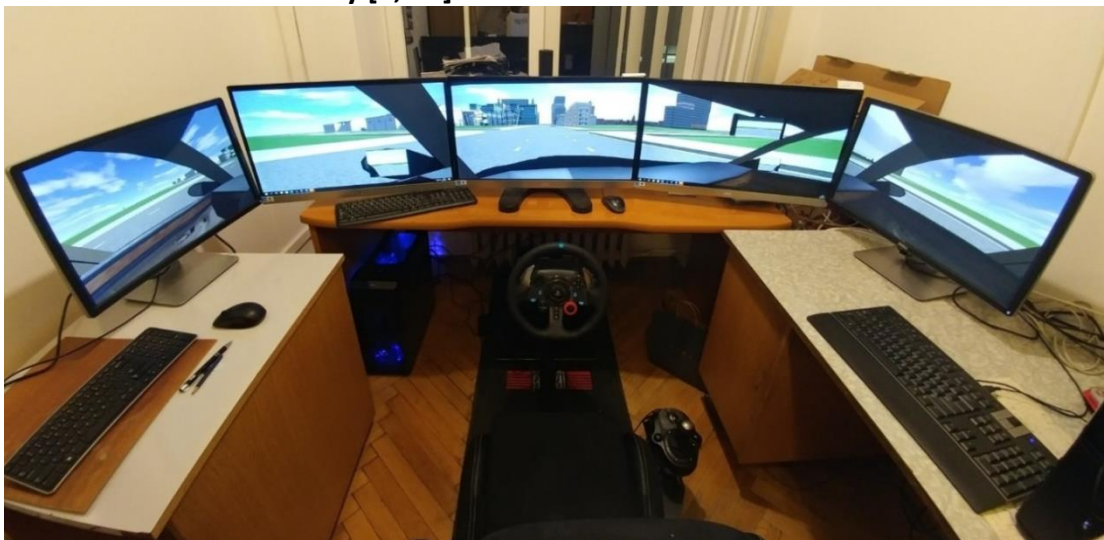
Mini-simulator stand for testing of Advanced Driving Assistance Systems (ADAS)
