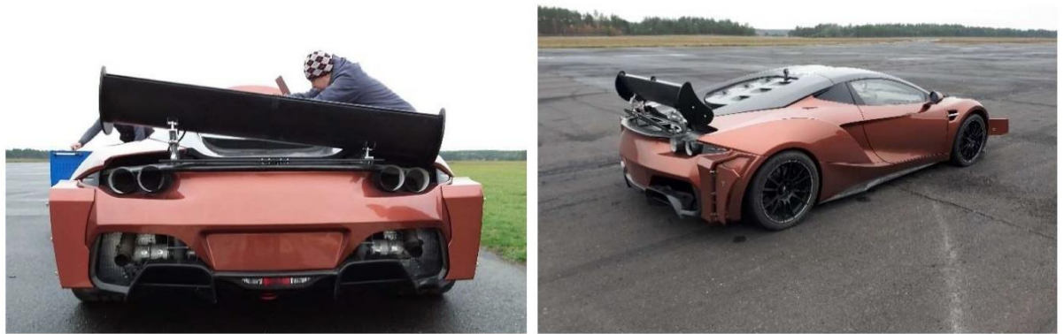
Photographs of the vehicle prepared for passage in two different configurations. Asymmetrically inclined wing for cornering configuration ( left ) and braking configuration ( right ).
