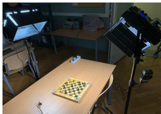
Fig. 7 Two LED lights and a camera — research on the influence of the light condition on object detection (source: Maciej Zieja, The chess pieces detection system of a robot for chess games in changing lighting conditions, engineering thesis, 2023)
