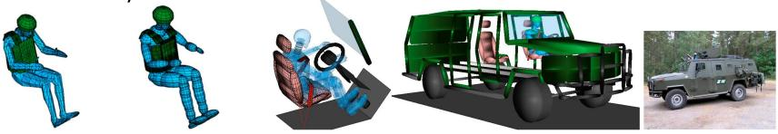
Experimental and simulation investigations and the assessment of improving possibilities of both crew safety and robustness of patrol and intervention vehicle when ramming into barriers
