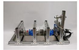
Testbed for Parallel-Series Elastic Actuators (PSEA)
