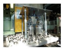
Self reconfigurable intelligent swarm fixtures for machining flexible aircrafts parts (implemented in Piaggio)
