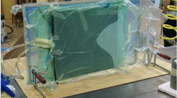
2. autoclave curing 270 min at 120°C, applied pressure 3 bar
