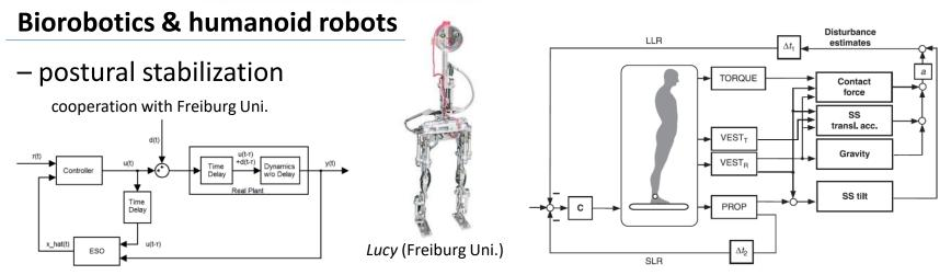
ADRC (Active Disturbance Rejection Control) vs. DEC (Disturbance Estimation and Compensation)
