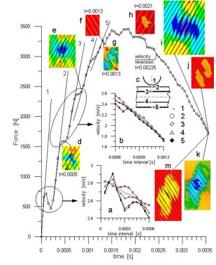
growth stages of delamination resulting from impact
