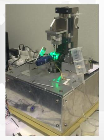
Artery mechanical properties testing machine
