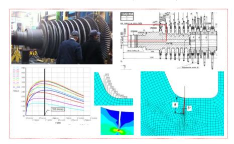
• FE ANALYSIS OF THE TURBINE BLADE LOCKING PIECE DEFECTS
