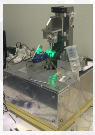
Artery mechanical properties testing machine
