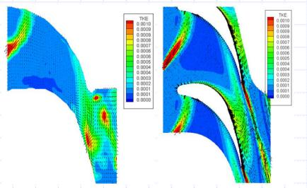
Flow with moving wakes (N3-60 profile). Contours of turbulent kinetic energy and perturbation vectors in the blade passage. left: experiment, right: simulation.
