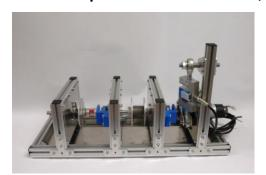
Testbed for Parallel-Series Elastic Actuators (PSEA)
