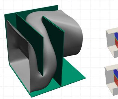
Optimisation of pressure loss in a flow around two obstacles
