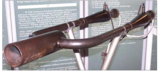
The Polish pulsejet engine from 1933. 1 – Air intake into the engine, equipped in an injector (a) and inlet valves; 2 – Combustion chamber with a spark plug (b); 3 – Exhaust pipes; e – Common propelling nozzle. Reconstructed on the basis of measurements made by Andrzej Glass
