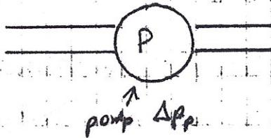
The micropump is used to maintain the Hagen-Poiseuille flow (laminar) in the pipe of the diameter  $\phi D$ .
