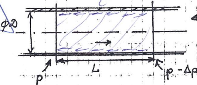
← stationary flow through the pipe segment. Find wall shear stress knowing  $\Delta p$ ,  $D$  and  $L$
