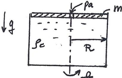
Floating flap with the mass m remains balanced by the fluid which rotates with the angular velocity  $\Omega$ . Find m knowing  $g, \rho_c, \Omega, R$ .
