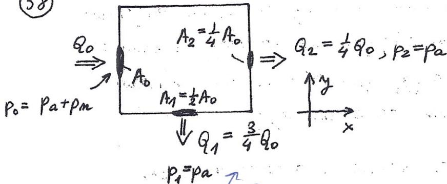
Find both components of the reaction ( $R_x, R_y$ )
