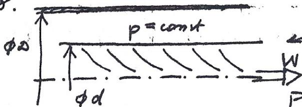
pipe with the solid core. The core is moving with the velocity  $W$ . Pressure is constant.
