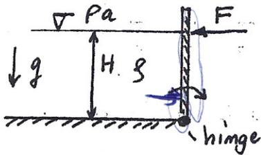
To keep the flap in vertical position the force F needs to be applied. Find the density  $\rho$ .
