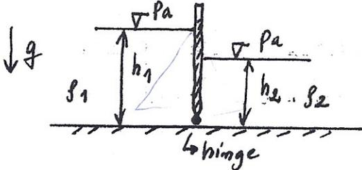
The flap remains in vertical position. The density ratio  $\rho_1/\rho_2$  is given. Find the ratio  $h_1/h_2$ .
