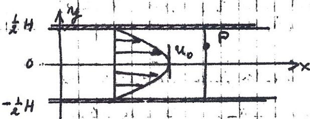
Poiseuille flow with the maximal velocity  $u_0$
