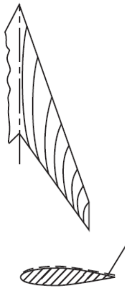
Attached flow with spanwise flow
