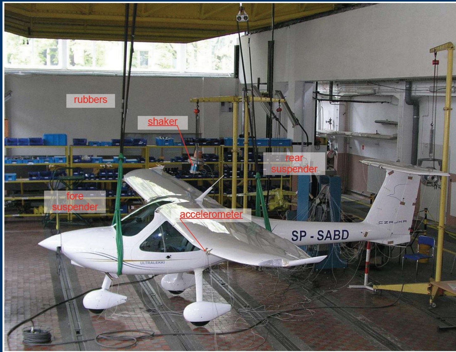
MP-02 „Czajka” UL-aircraft during GVT
