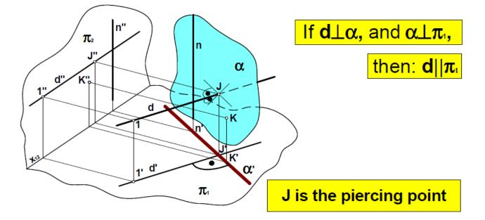
The point **J** is the point of intersection of the plane  $\alpha$  pierced **by** the straight line **d**, what can be marked as;
